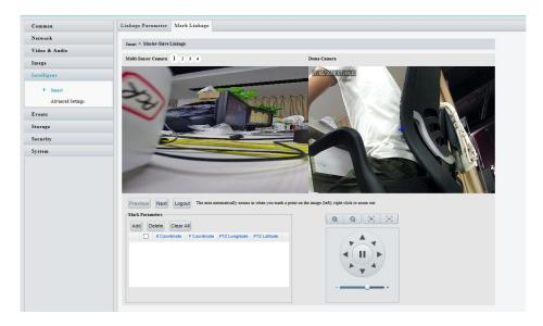
**10.** Marking steps on a single scene: Click **Add**, click on the left master camera image. A small white frame appears at your clicking, and the area automatically zooms in (as shown below). Adjust the position of the marking point on the enlarged area. Right click to return to original image and select again. Click **OK** to confirm current marking point.
