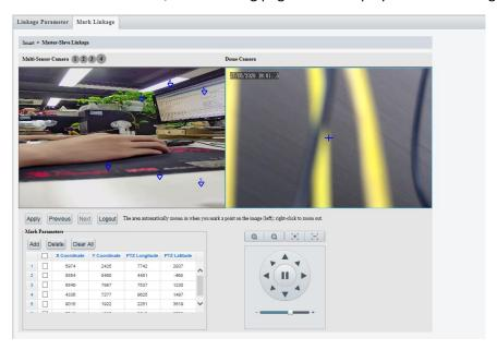
OK/Apply: After completing the marking of one scene, click **OK** or **Apply** to save and update the linkage between the master and slave camera.
